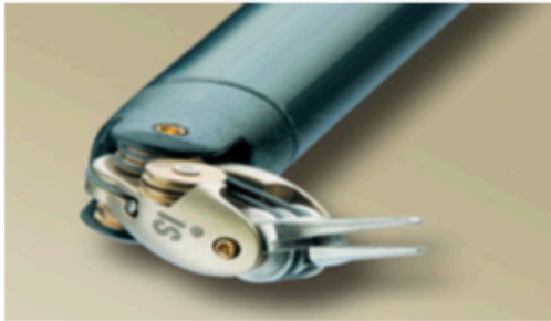
Picture 4 - Endwrist function of the 8mm robotic instruments
