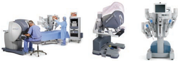
The 3 components of the robotic system: Surgeon console, patient cart and tower.
